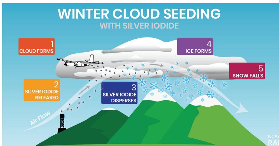
Ground-based generators and/or aircraft are often used to disperse AgI into the clouds.
