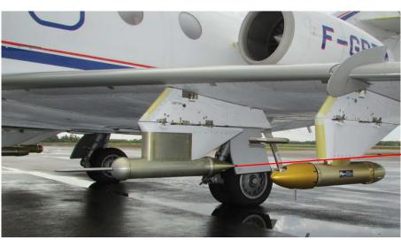
Erosion damage - radome, wing tip, & LWC sensor
