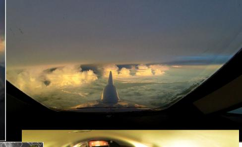
FS140018 - 3.4 F/H – Flight in system located North/West of Broome. 6 legs performed at FL310 / - 30°C with sustained IWC at 1.0g/m3 and peaks from 1.5g/m3 to 2.5g/m3 (1 peak).
