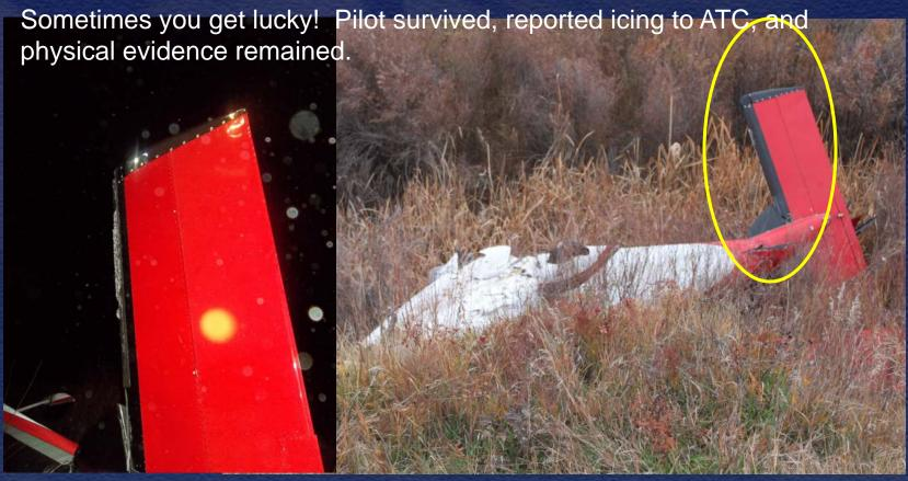
NTSB Probable Cause: The pilot's improper decision to continue flight into known icing conditions, which adversely affected the airplane's performance and resulted in a loss of airplane control.
